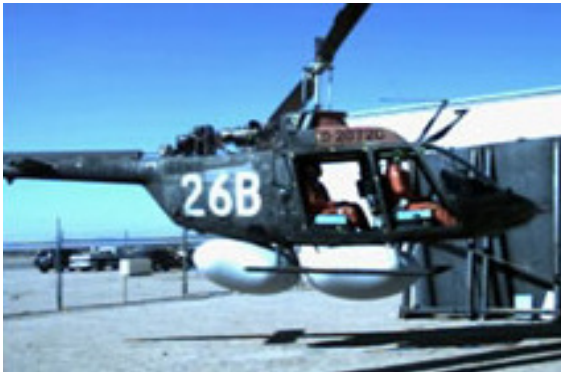
Israeli Bell 216 equipped with airbag for emergency landing
