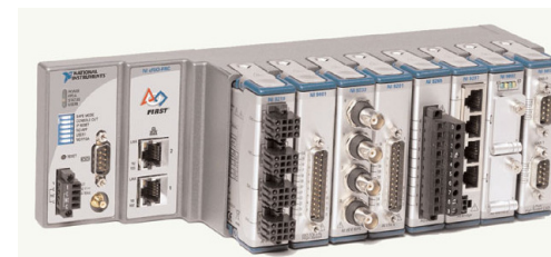
FPGA control unit cooperating with Labview system
