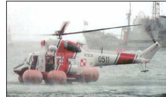
Polish helicopter Anakonda equipped with airbags for landing on water
